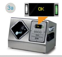
If the container content is identified as conforming, the "OK" message and a green light are displayed.
